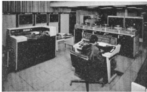
Figure 5. The CDC 3300 at ICA's headquarters (circa 1970). The punched-card reader and magnetic-tape units are to the left, with removable disk units toward the back. Curtains in the front and back of the building were drawn to help control the temperature. Toward the top there is a glimpse of the mezzanine floor housing programmers. (Courtesy of Fundación ICA.)
